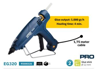
Professional and universal glue gun with compact size. Comfortable to operate and designed for precision work, even in intensive use. Comes with fixed and adjustable stand for versatility, fast warm-up time, interchangeable nozzle and a glue output of 1,000 g/hour.
